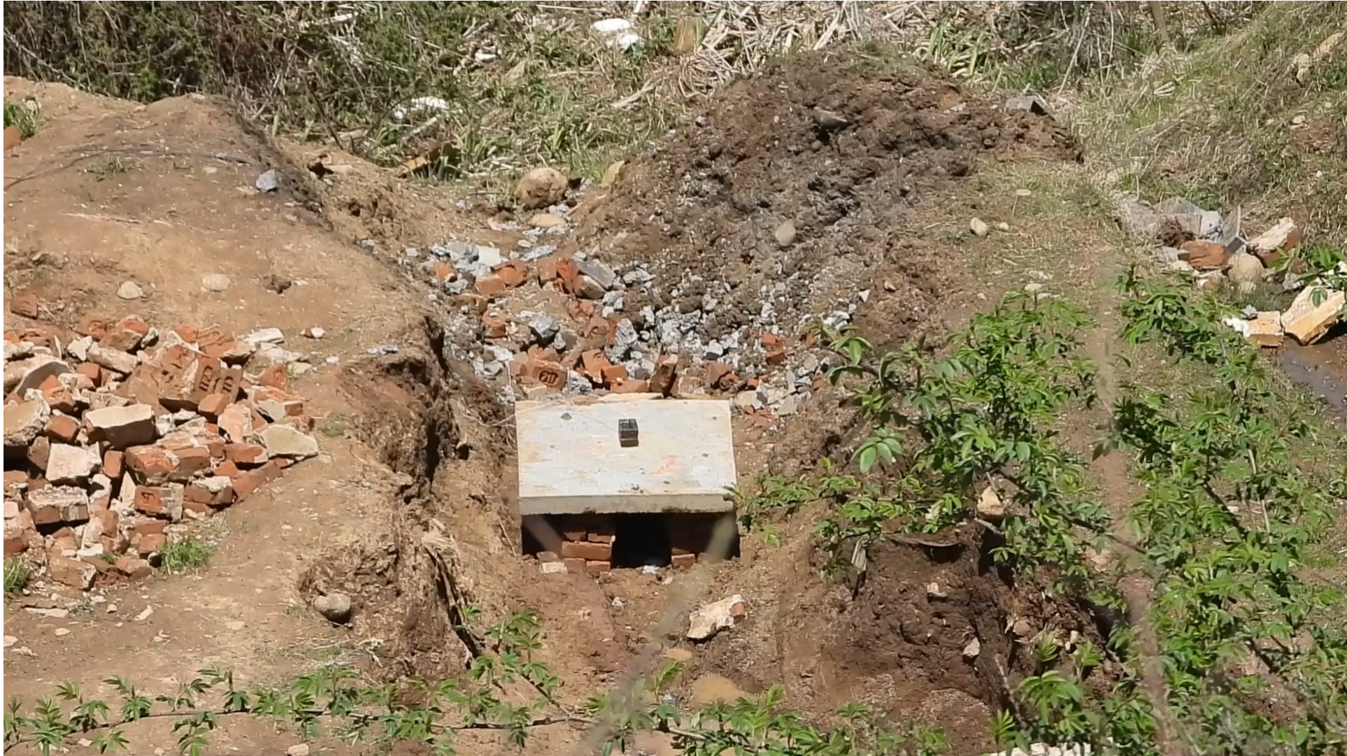
Field test of BFRP reinforced concrete (RC) panel subjected to 1.35 kg TNT charge weight under contact blast
