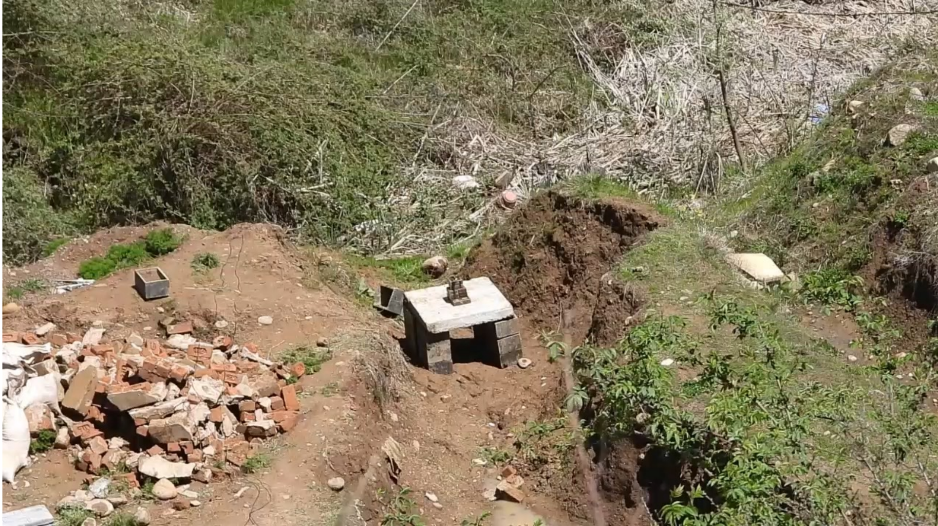
Field test of BFRP reinforced concrete (RC) panel subjected to 4.5 kg TNT charge weight under contact blast
